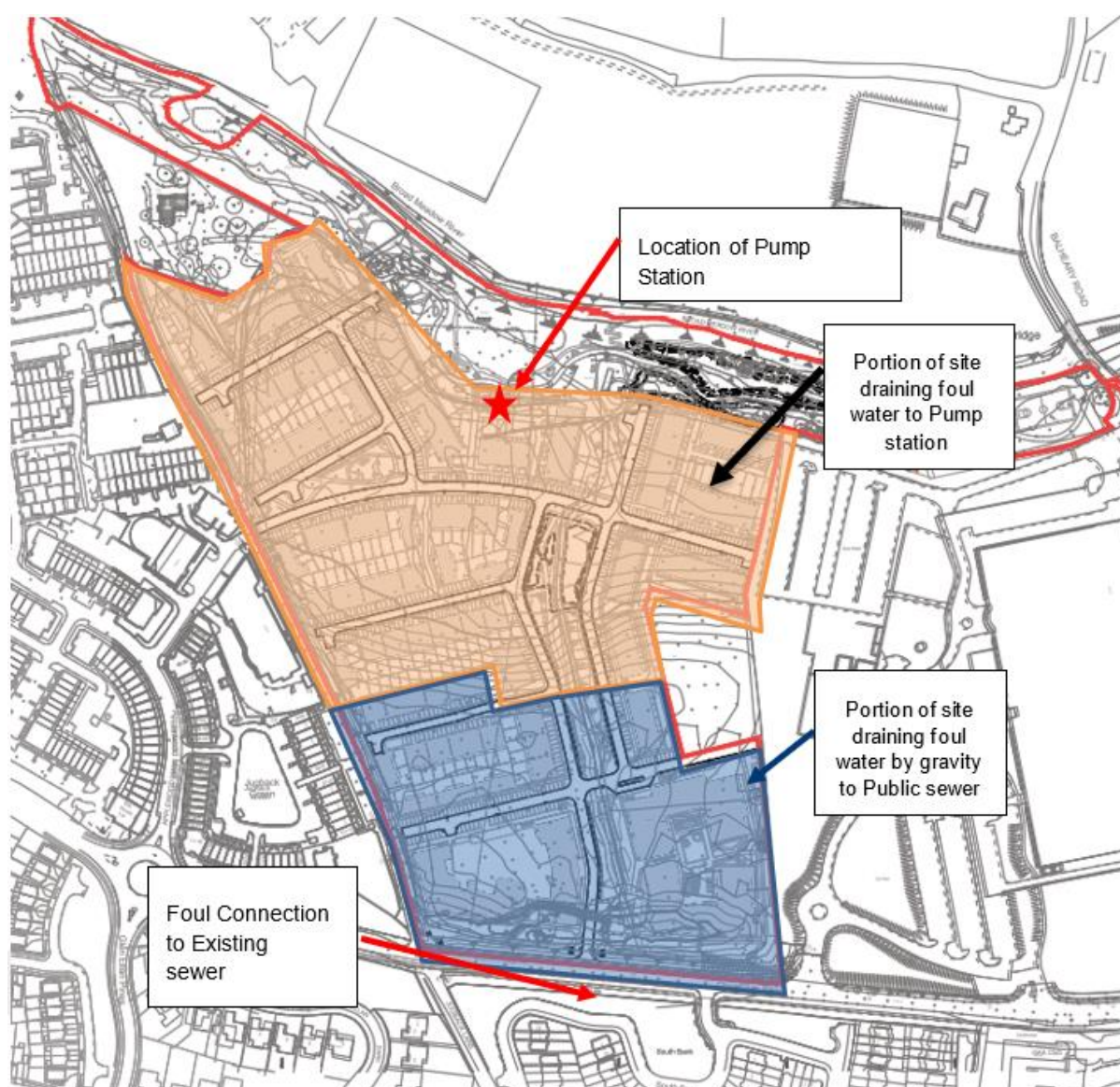
Figure 15.3 Foul Water Scheme
